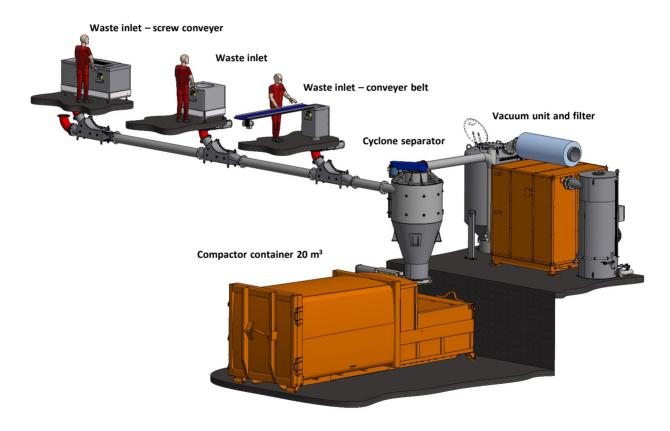
**Improved logistics and profitability, lower processing costs.** No more need to move waste and by-products through the production area in bins. No more load peaks, as the vacuum system feeds material in even batches, leaving the area free
